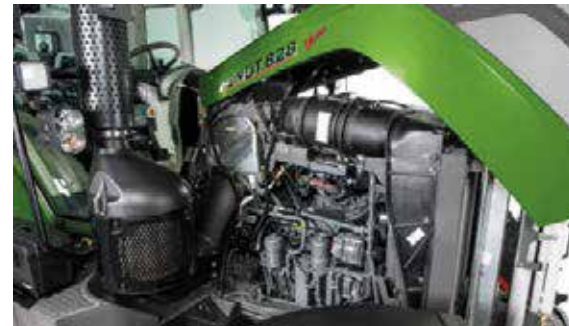
A swing-up bonnet and easily removable side panels provide excellent access to the engine compartment.
